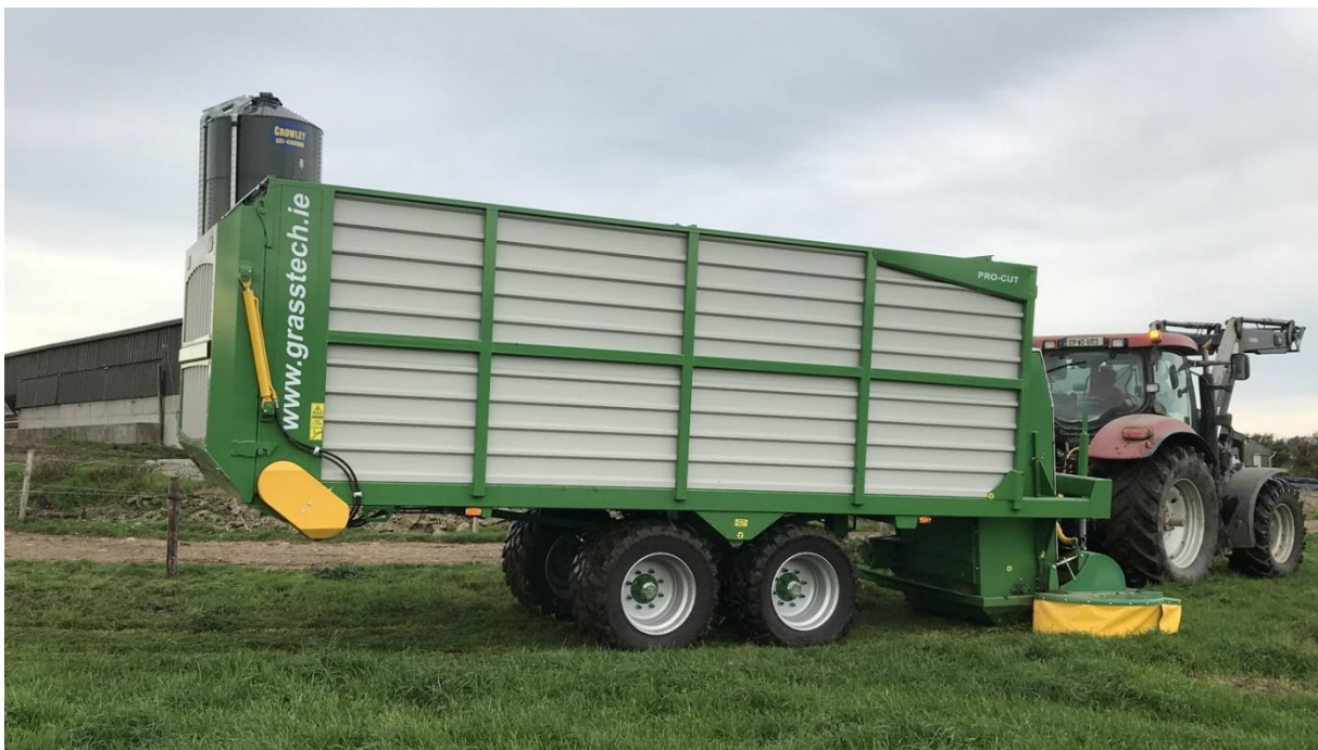
Figure 12. Combined mowing and harvesting equipment used in the Danish DEMO (grasstech gt-140) (source: Grasstech.ie).
