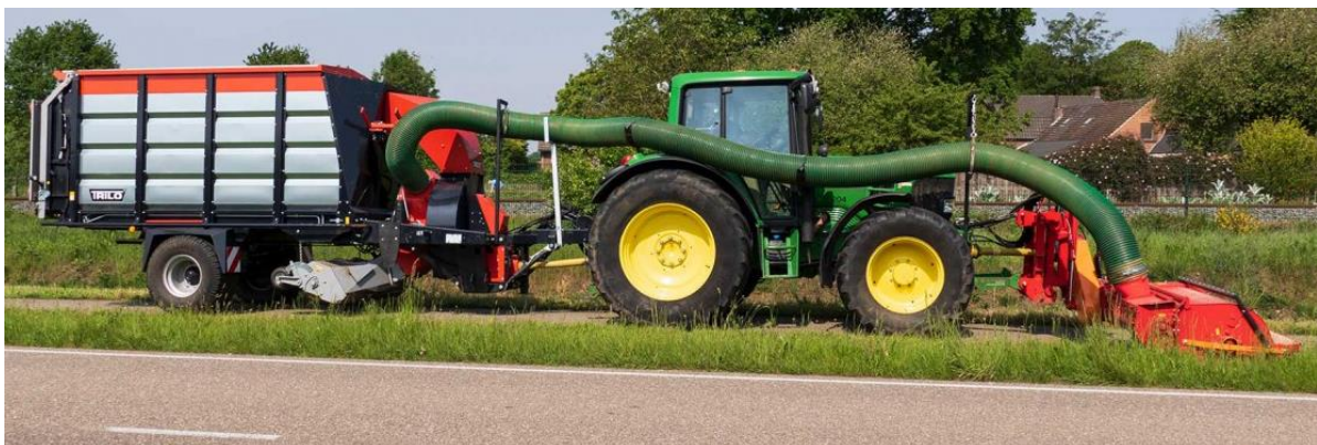
Figure 8. Trilo S10 suction wagon with a separate flail mower in front of the tractor. The grey bar underneath the suction wagon can be replaced by a flail mower, creating a single device for cutting and collecting (source: Trilo).
