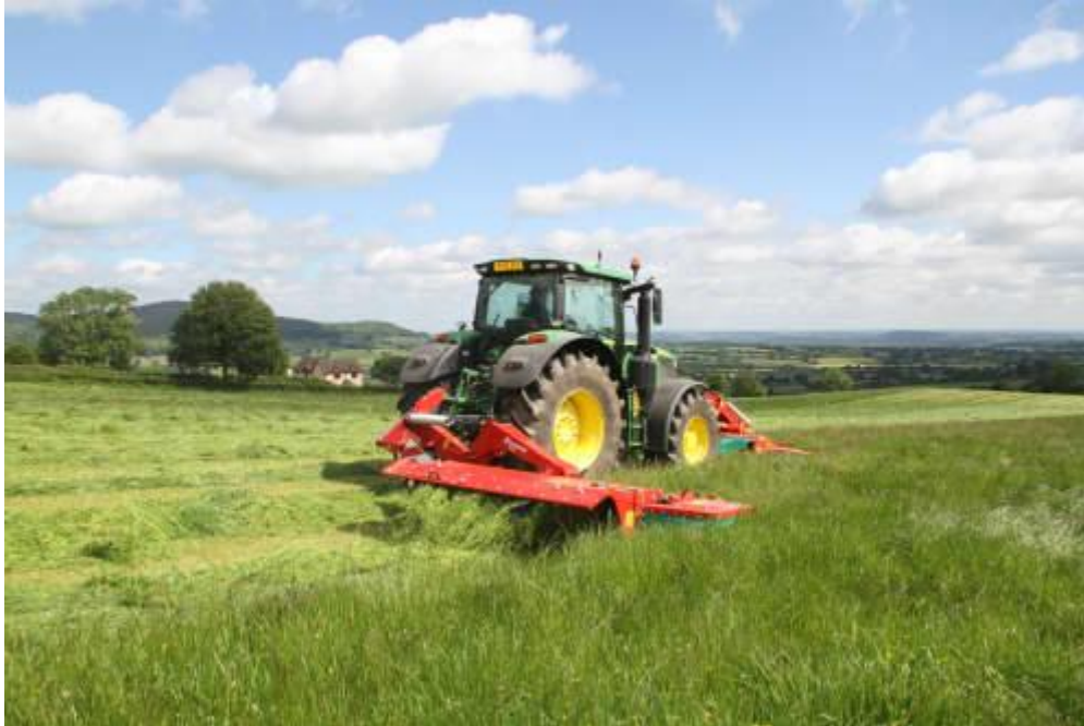
Figure 13. Large-scale Kverneland 3232 MN disc mower (source: Kverneland).
